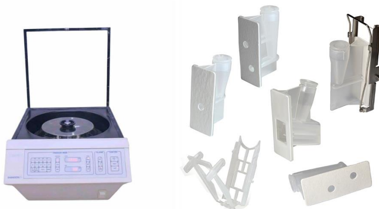
Figure 7: Image of the Cytospin machine and the cytofunnel-slide setup.
