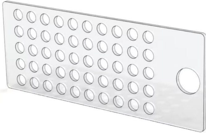
Figure 8: Image of the cell gasket used in fixation experiments.
