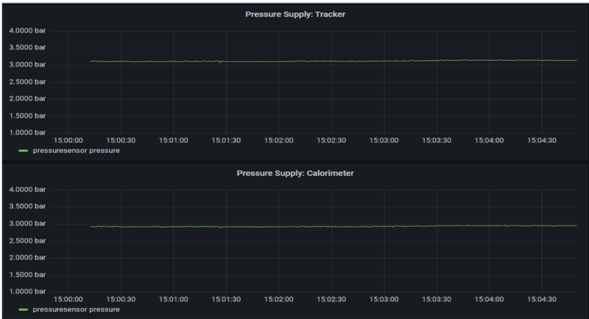
Figure 20: Grafana example of two separate graphs. Grafana allows for displaying data from any given sensor with chosen axis labels. Graphs can be organized on the same plot or separated at will.
