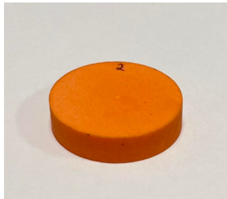
Figure 3.1: Apex R3 matching layer with nominal dimensions 20.14 \text{ mm} \times 4.9 \text{ mm}
