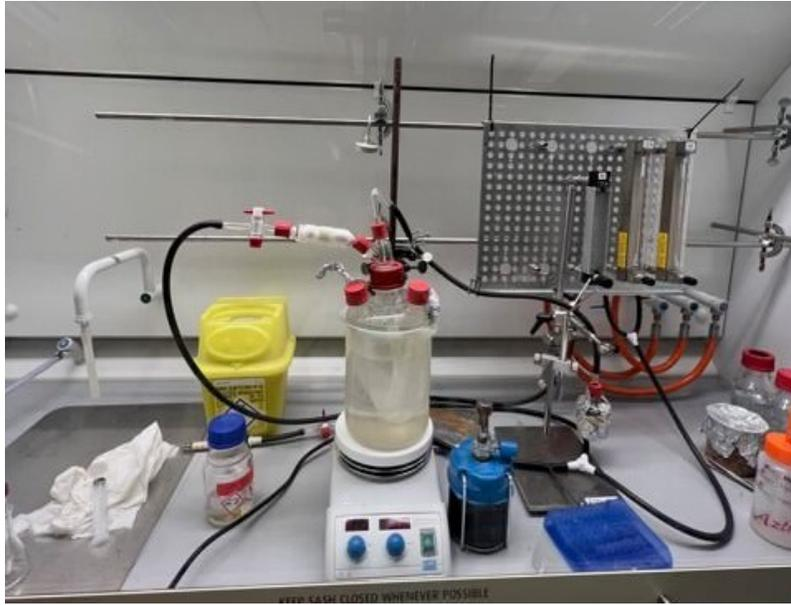
Figure 3.3: The experimental setup for preparing media under the fume hood.
