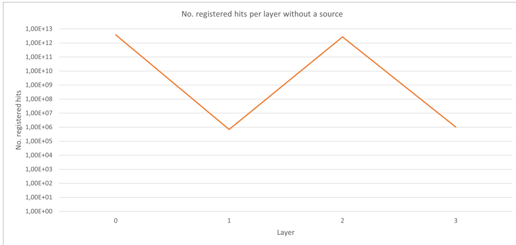
Figure 5.7: Number of clusters per layer of the mTower registered by the ALPIDEs from cosmic muon detection. For layer 3, the number of hits is multiplied by 2.
