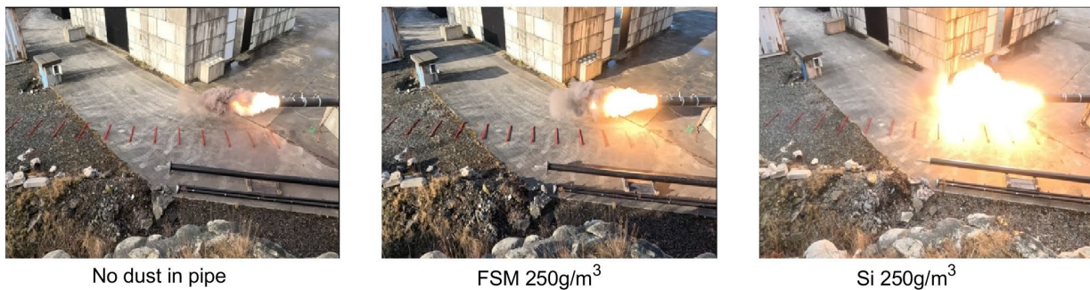
Figure 31: Comparing fireball size in configuration 1 for 250g/m 3 of Si and FSM with no dust in pipe.
