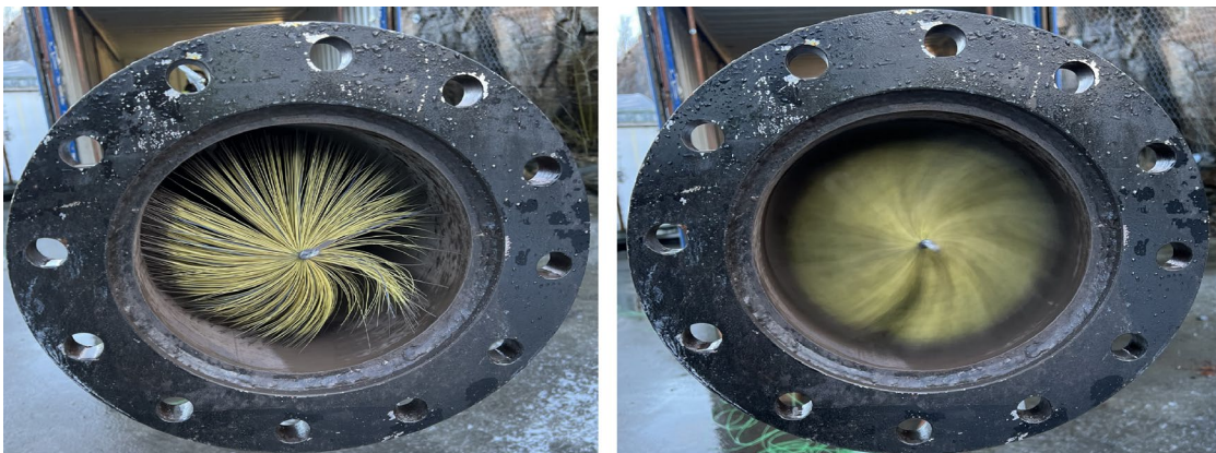
Figure 23: Illustrating the rotating cleaning brush in DN250.
