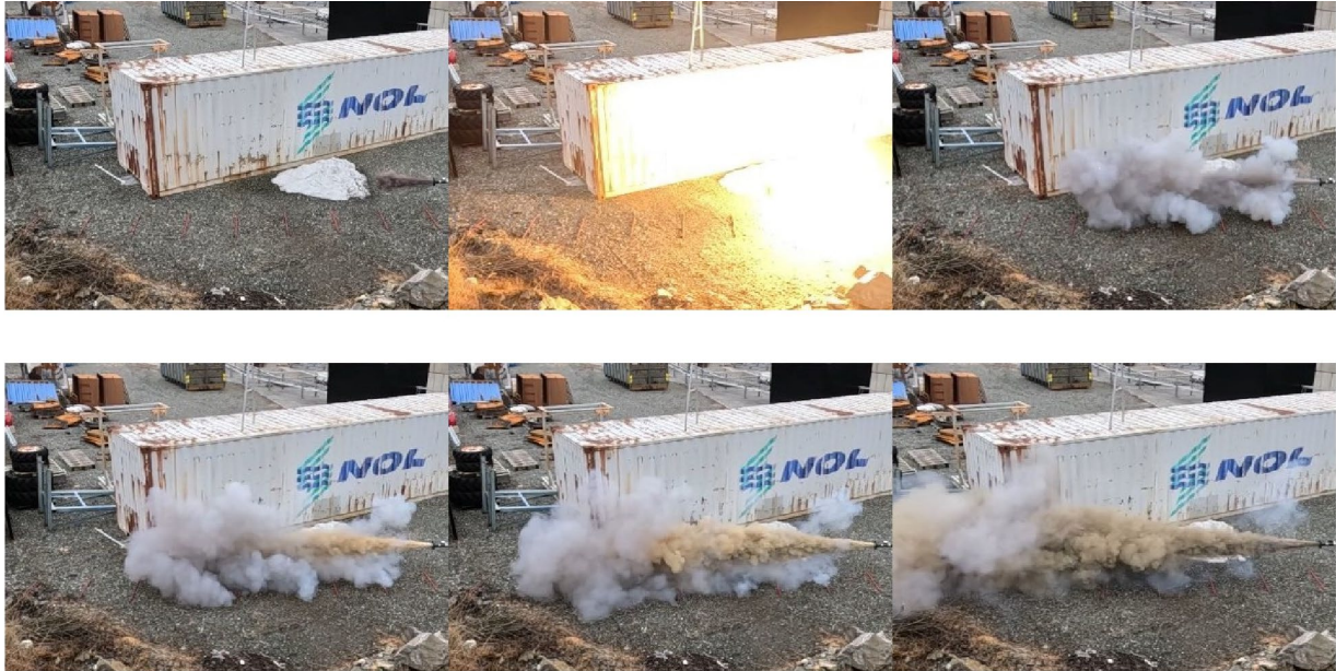
Figure 46: Dust cloud observed in Test #1 with silicon in configuration 6.
