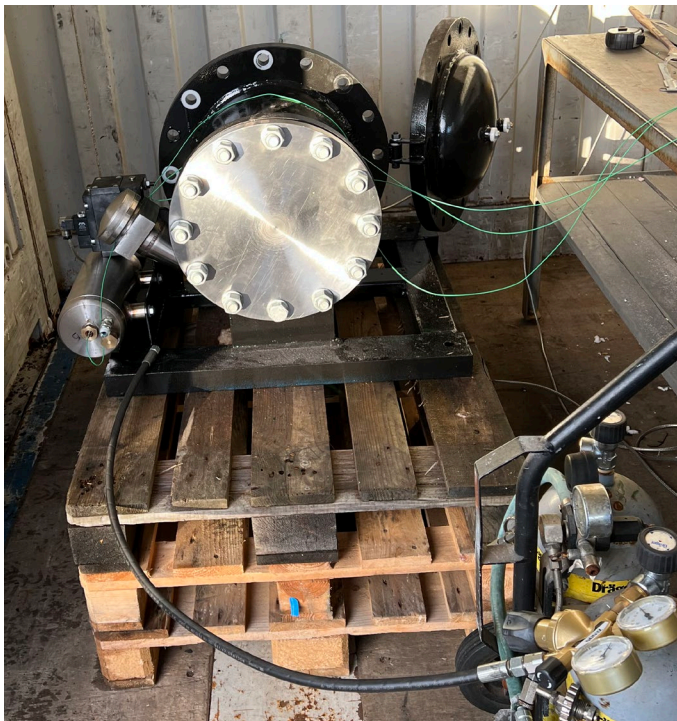
Figure 20: 32-litres ignition Chamber with blind flange
