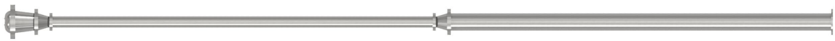
Figure 58: Illustration of configuration 4, which comprises a 6-metre DN160 pipe and a DN250 pipe.
