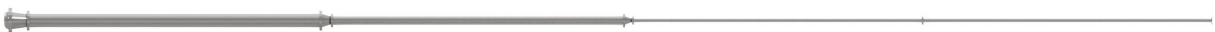
Figure 60: Illustration of configuration 6, which comprises a 6-metre DN250 pipe, a DN160 pipe, and two DN60 pipes interconnected with crossovers.
