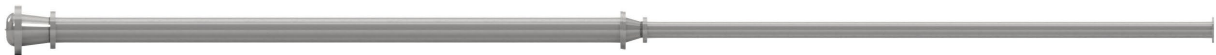
Figure 57: Illustration of configuration 3, which comprises a 6-metre DN250 pipe and a DN160 pipe.
