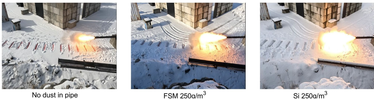
Figure 36: Comparing fireball size in configuration 2 for 250g/m 3 of Si and FSM with no dust in pipe.
