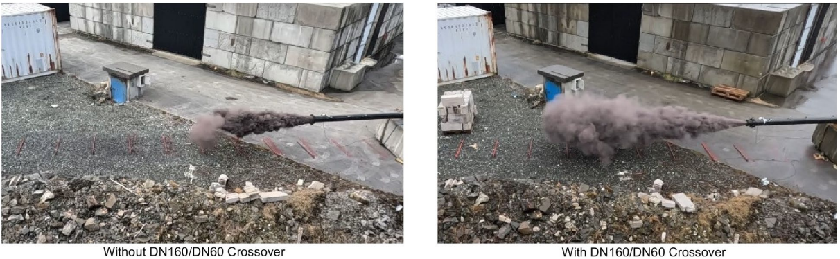
Figure 44: Comparison of dust cloud exiting the DN160 pipe with and without DN160/DN60 crossover.
