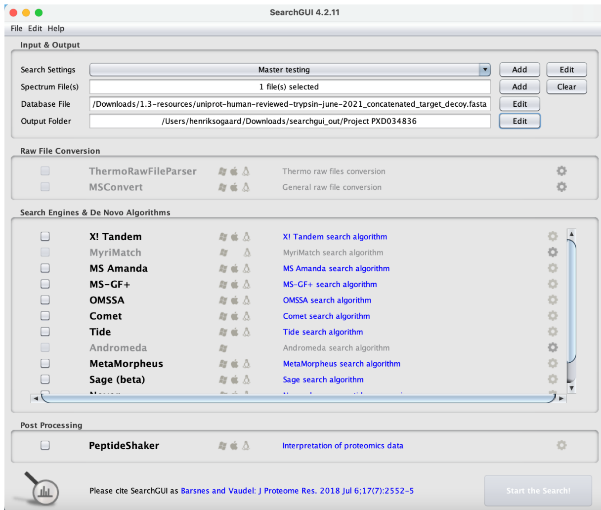
Figure 11: Screenshot of SearchGUI. The greyed-out proteomics search engines are search engines that cannot be used on the current operating system.
