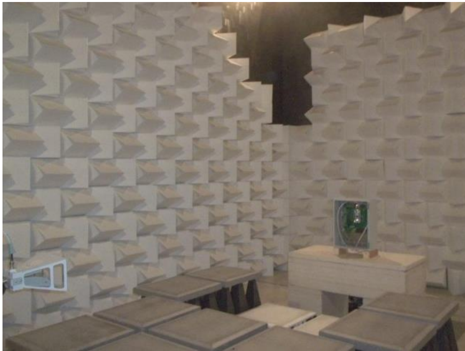
Figure 0-2: Test Setup Radiated 1GHz and Above [19]
