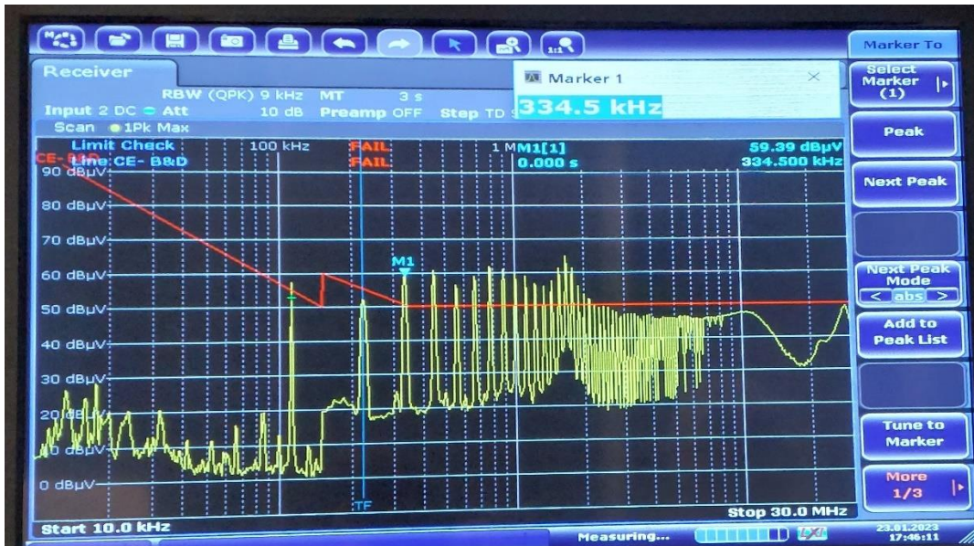
Figure 5-8: Conducted Emissions Failure (10KHz-30MHz)
