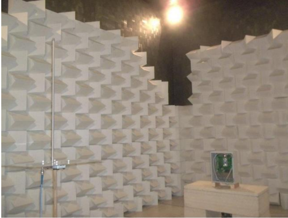
Figure 0-1: Radiated Emissions Test Setup (150KHz-30MHz) [19]
