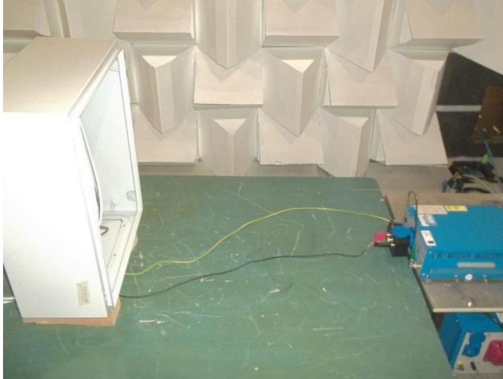
Figure 5-3: Test Setup Conducted Emissions [19]
