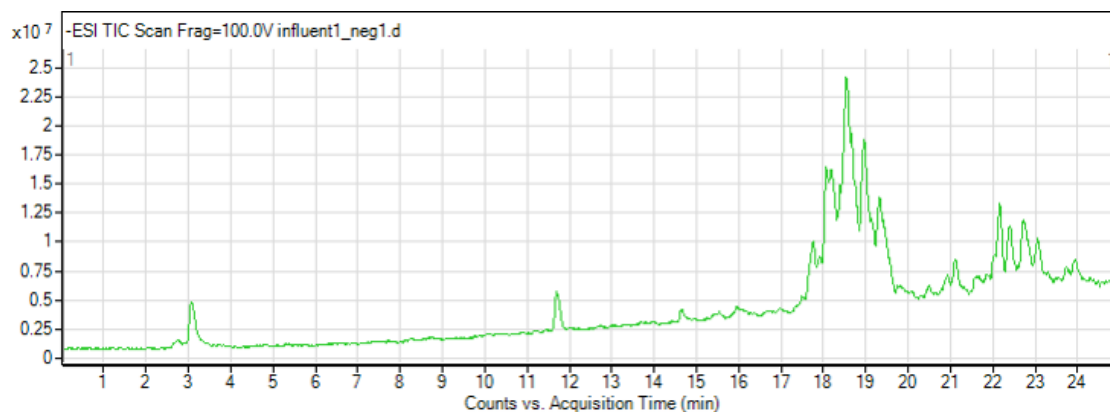
Figure 62: Total ion chromatogram of the sample called "November, Influent1_neg1" in the negative ionisation mode.
