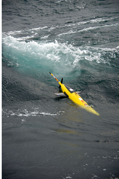
Figure 3.3: Deployment of a Kongsberg Seaglider. Photographer: Rudi Jozef Maria Caeyers
