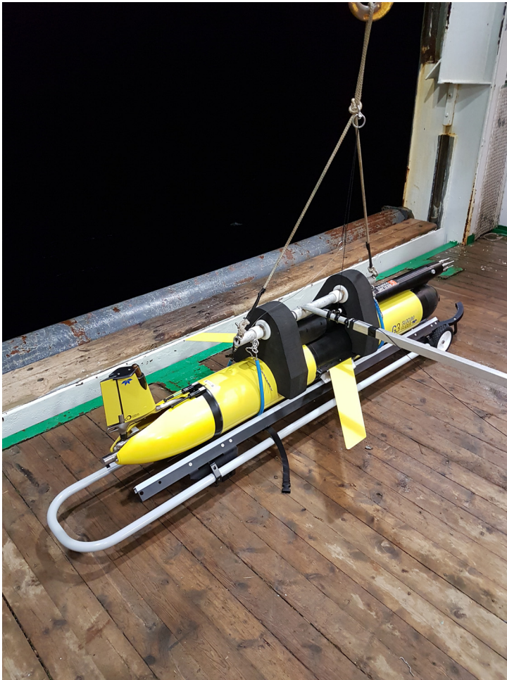
Figure 3.5: Slocum glider Odin with MicroRider ready for deployment
