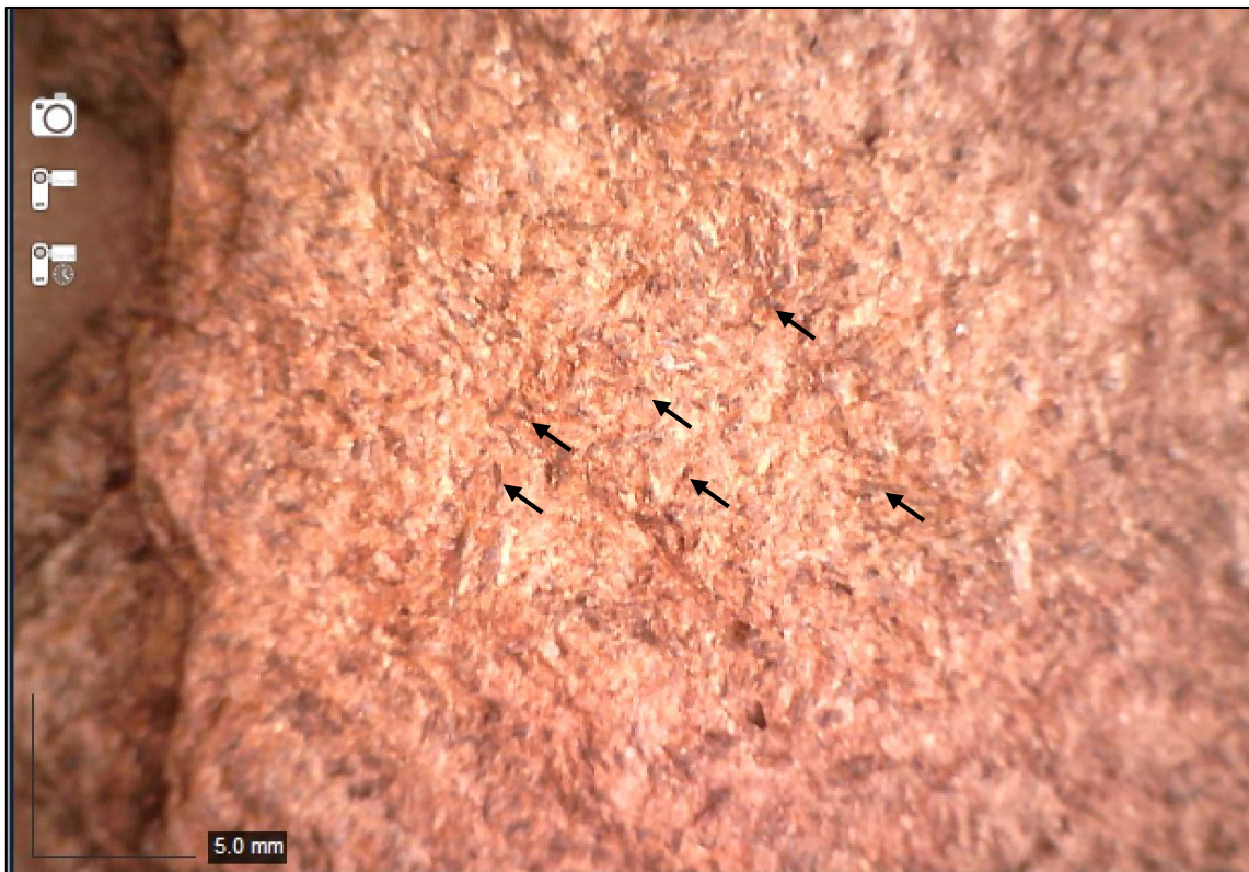
Figure 2.1.2: Bakestone BRM1/2363/9 of medium-grained chlorite schist. A few of the visible amphiboles are pointed out. 10x magnification, microscope picture by MFE 2023
