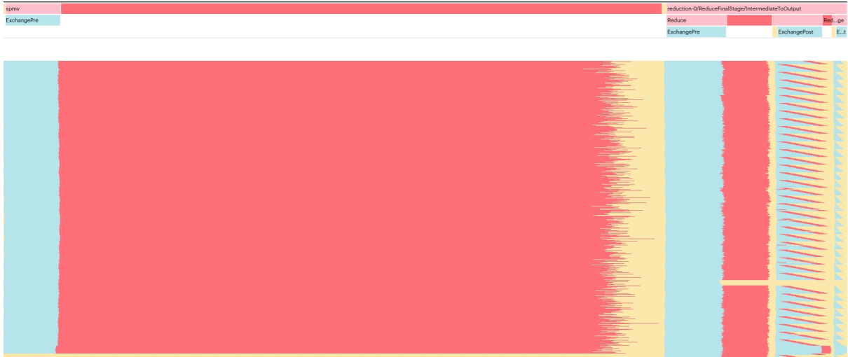
Figure 4.1: A flame graph of the SpMV algorithm while executing bfly.mtx (1-round). Each line represents a single tile on the IPU
