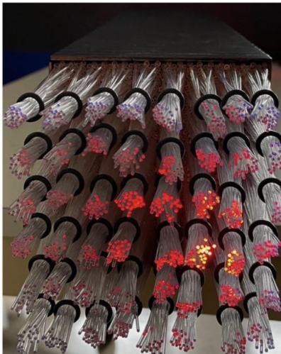
Figure 2.2: The scintillation fiber bundles for the FoCal-H prototype used in the 2021 test beam.[11]
