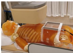
Figure 13: Impact of an X-ray blanket on patient dose. To assess the increase in dose rate below the X-ray blanket, a bi-directional DAP meter was attached to the abdomen of the X-ray phantom. Measurements were repeated with and without an X-ray blanket. The upper panel illustrates dose rate according to presence of X-ray blanket and the lower panels show the experimental setup.
