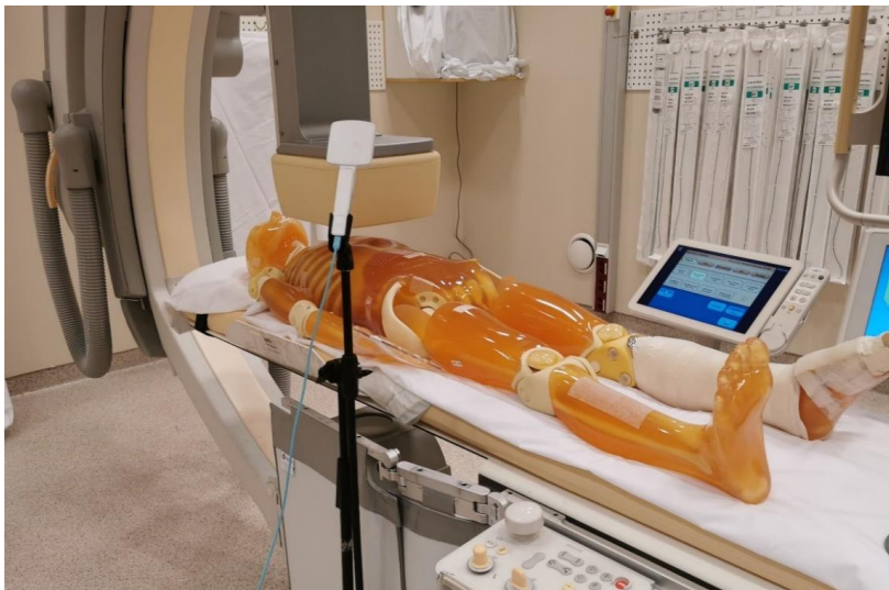
Figure 11: Bench testing setup. An anthropomorphic X-ray phantom is used to simulate the patient in the cath lab. Scatter radiation is measured with the X2 survey sensor (Unfors Raysafe AB, Sweden)
