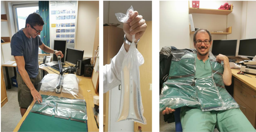
Figure 21. Manufacturing a sterile plastic cover for the FMX. In the left panel, an image of the welding machine used to produce the prototype of a plastic cover. The welds were checked for solidity and sealing with water (middle picture). To the right is the FMX with its plastic cover.
