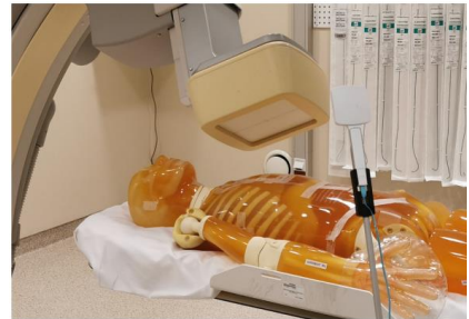
Figure 24: Bench testing setup for measuring scatter radiation to the operator. An anthropomorphic phantom was used to simulate the patient. The C-arm is in LAO-CRAN projection.
