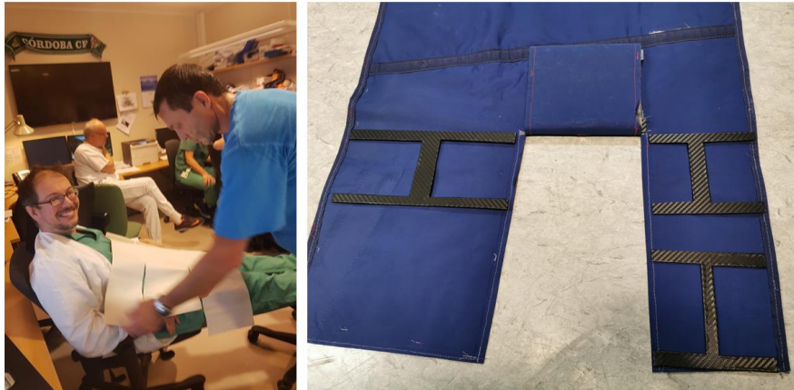
Figure 18: Early prototypes of the FMX. The left panel is a picture of the three-flap configuration with a prototype made of paper. The right panel shows the first working prototype. To improve stability and ease of use, we experimented with a variety of battens in different configurations.
