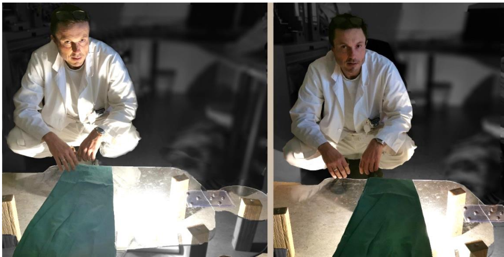
Figure 10. A simple visible light model to illustrate scatter radiation. To the left the X-ray blanket is positioned too far towards the patient's legs. In the right picture the operator is protected in the shade of the X-ray blanket.
