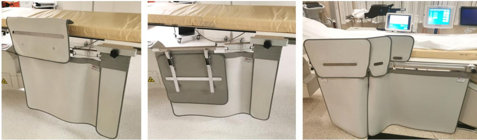
Figure 4. Table-mounted shield designs. In the left panel a smaller model is shown. Width and length are limited and there is a single top shield. In the middle panel, the top shield has been flipped down, which leaves a large unshielded area. To the right is a newer model with three top shields, and a wider under-table shield that extends protection to the second operator or nurse.
