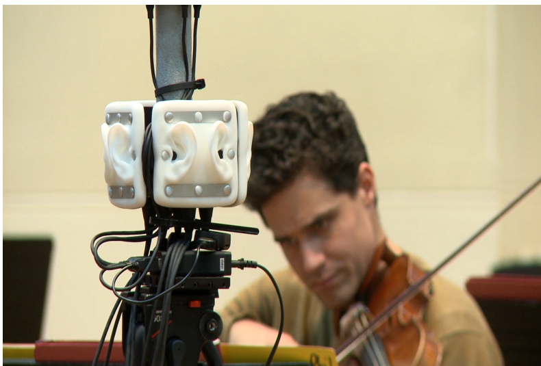
Figure 1.1: Screenshot from Philharmonia Orchestra’s video [1] about their VR experience, showing the Omni Binaural Microphone [2], made by 3DIO [3], that they used to record the audio.
