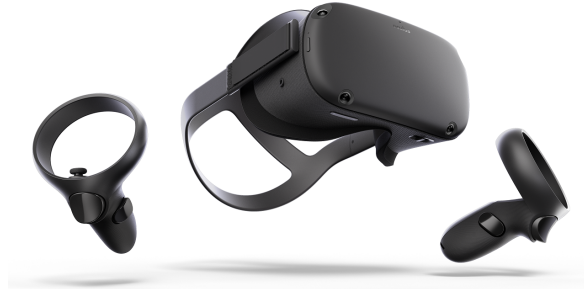
Figure 2.8: The Oculus Quest [16], a standalone VR system running on mobile hardware and Android.
