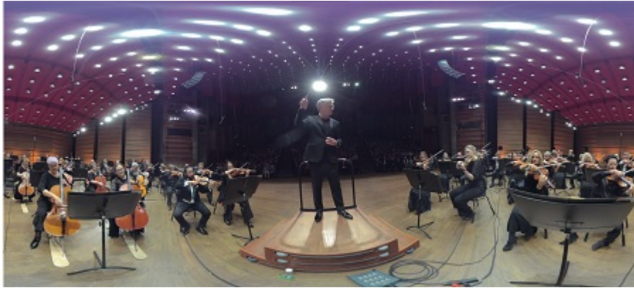
Figure 3.13: What the 360° video looks like when playing in a normal video player, as it is formatted using equirectangular projection.
