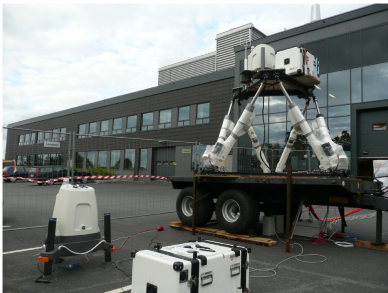
Figure 6.1: Setup of lidars on motion platform and the reference lidars in 5 m horizontal and 3 m vertical distance on the ground at the Grimstad campus of the University of Adger, Norway. Picture imported from the experiment report (Hellevang et al., 2012)
