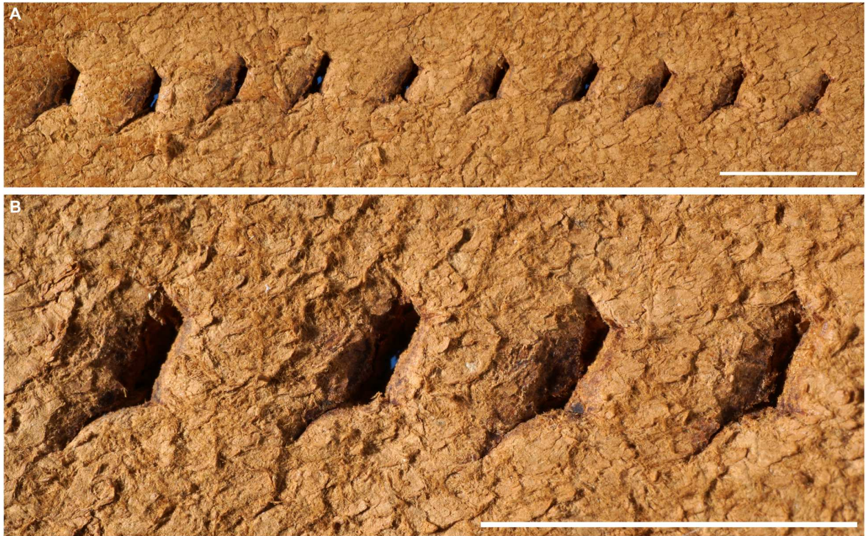
Fig. 7. Leather pricking experiment. Series of perforations made into thick leather using a burin as a stitching chisel and a short rib as a leather punch board (A) and close-up (B). Scale bars, 1 cm.
