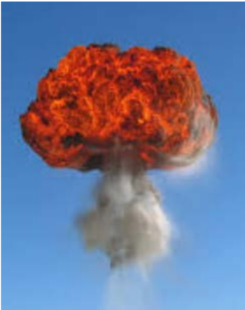
Figure 18 BLEVE fireball; spherical when fully developed
