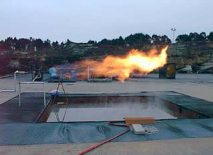
Figure 1 0.3 kg/s jet fire. Propane vapour jet. Flame length is 6-7 m. Upstream pressure 11.5 barg and 16 mm nozzle. Picture is taken from PhD report by Leiv Anfin Drange
