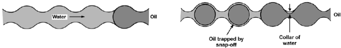
Figure 2.5: Trapping in a Snap-off model [9].
