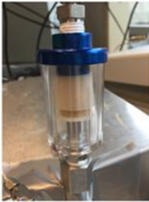
Figure 3.1.3a: Moisture trap to the left. Schematic of moisture trap placement to the right.
