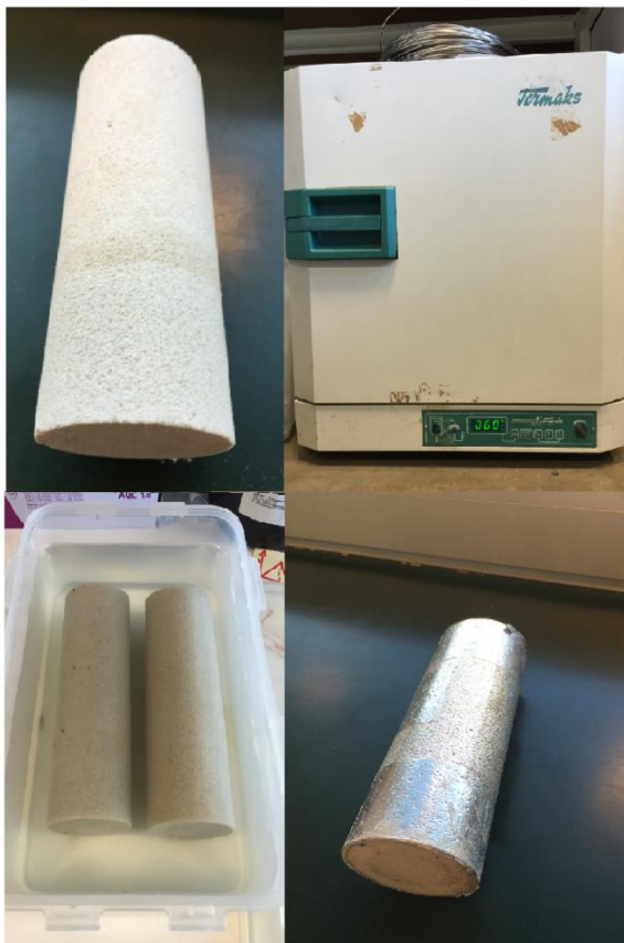
Figure 3.1.4: Bentheim sandstone core (upper left). Heating cabinet (upper right). Two cores during saturation (lower left). Core wrapped in aluminium foil (lower right).
