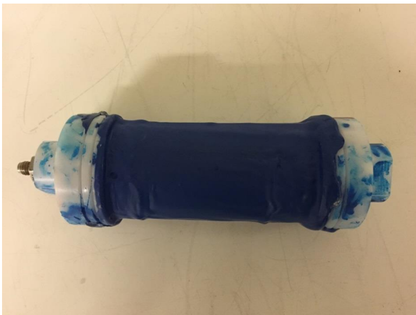
Figure 3.2.2: Sandstone core fitted with end-pieces and covered with epoxy.
