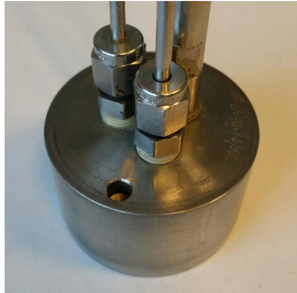
Fig 3.1.2b – (Left) shows the side of the end piece that is in contact with core on the inlet side in setup C. The three circular openings are channels that connect the core with the pump or a thermometer. (Right) shows the other side of the end piece on the inlet side in setup C. There are two 1/8 inch swagelock tubes that is connected to the end piece channel. The last channel is not used.
