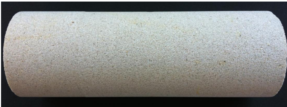
Fig 3.1.4 – Bentheimer sandstone, cut to approximately 15cm in length and 5cm in diameter (Hågenvik, 2013).
