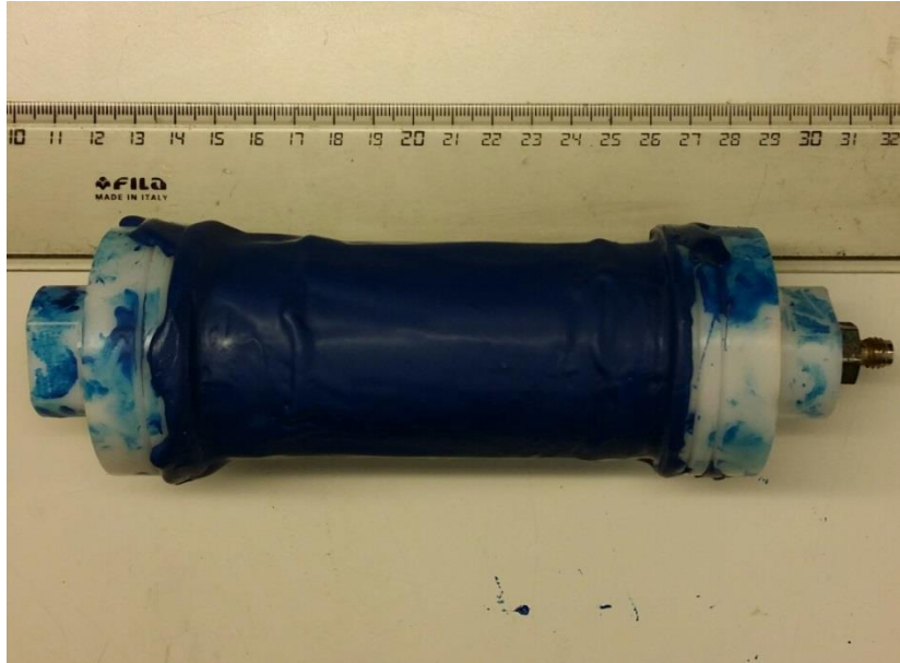
Fig 3.2 – A Bentheimer sandstone core sealed fitted with plastic end pieces and covered in epoxy glue. The scale in the picture is in cm.
