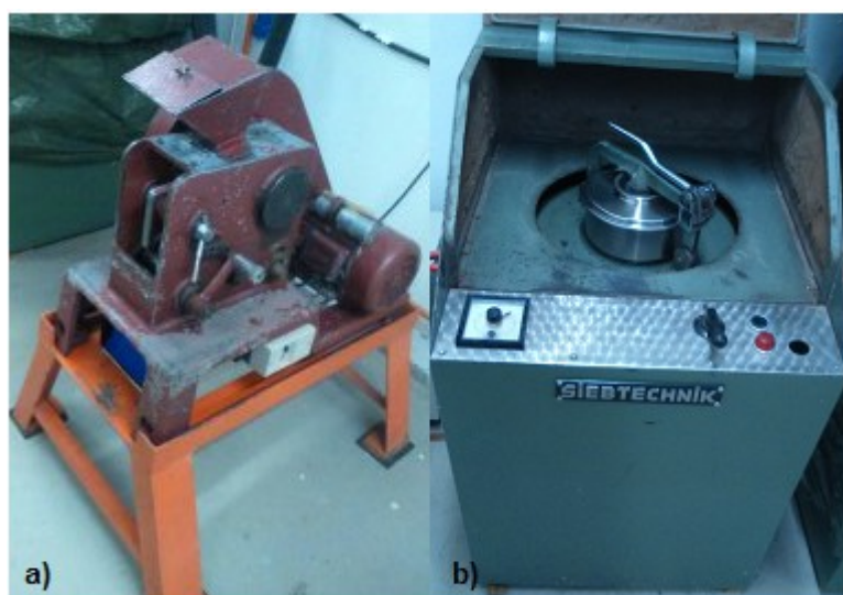
Fig. 3.1. a) Jaw crusher located in the basement in UiB.
