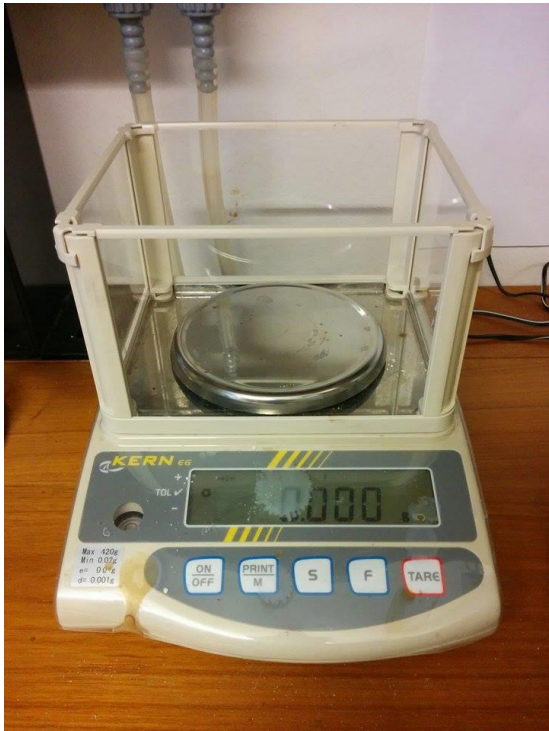
Figure 2.7: Precision mass balance used for water mass determination.
