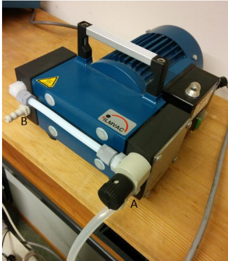
Figure 2.4: The ILMVAC two way compressor showing A) the intake port (used to create vacuum) and B) the outlet port (used for clearing the hydrate cell of residual water and gas between experiments).
