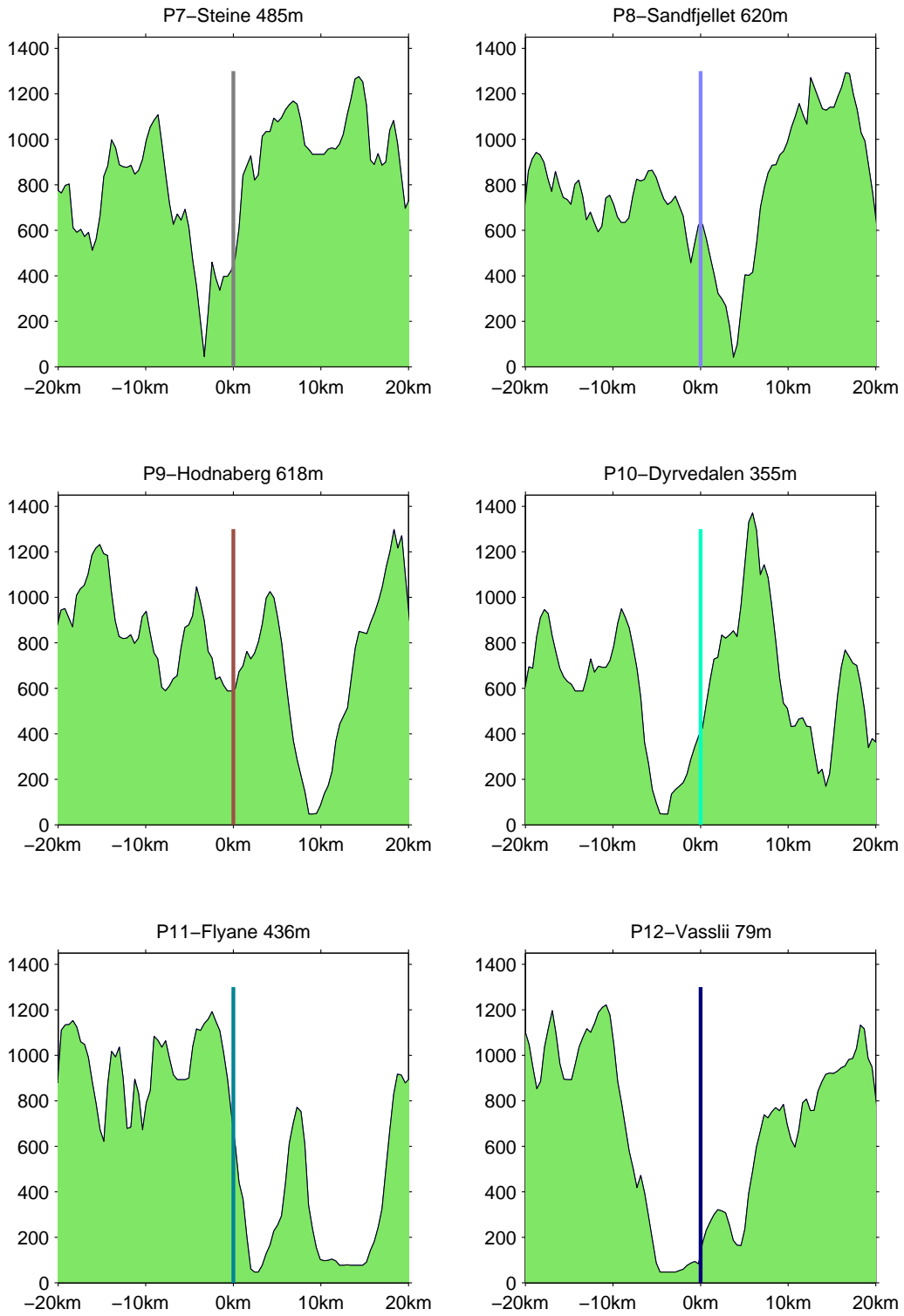
Figure 5.12: Terrain profiles for stations P7-P12, direction is 220°.
