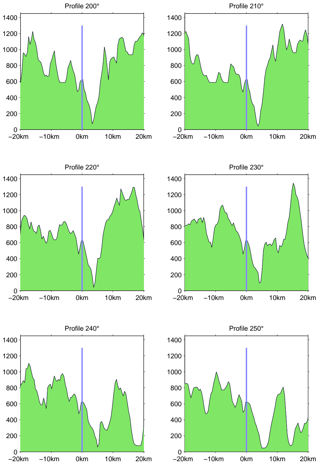
Figure 5.9: Terrain profile from P8, Sandfjellet. The panels corresponds to wind directions from 200° to 250°.
