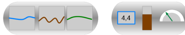
FIGURE 2.6: Real-time process visualization trend lines, with three different display types for the current value. Current values and recent history is easily visible, but deeper relationships between parameters are hidden. Image courtesy of Braseth et al. [7]
