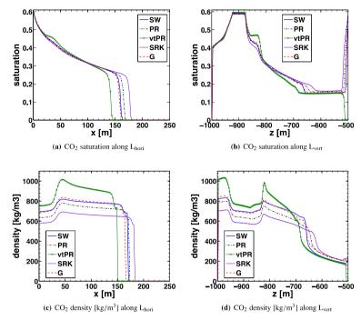
Fig. 6. Simulation results after 30 days of injection: Comparing the different cubic EOS against SW.
