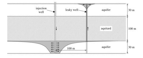
Fig. 4. Leakage scenario in 3D reservoir.
