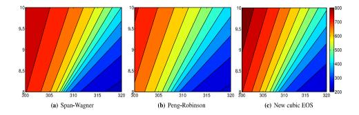
Fig. 1. Isochores [kg/m<sup>3</sup>]. Pressure [MPa] (vertical axis), Temperature [K] (horizontal axis).
