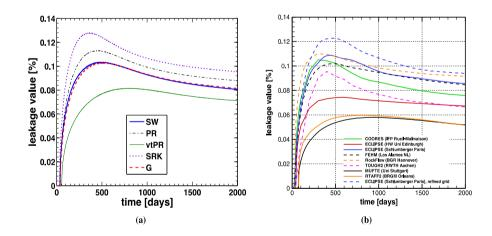
Fig. 7. (a) Results of Simulation 2. Comparing simulation results for the different cubic EOS for CO2 against SW. (b) Simulation results from [5].
