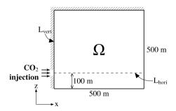
Fig. 3. The 2D reservoir domain of Simulation 1.
