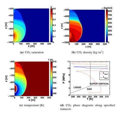
Fig. 5. Simulation results after 30 days of injection.
