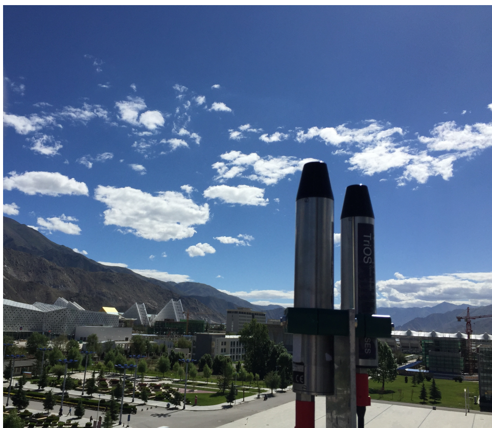
Figure 3.9: TriOS Ramses-ACC-VIS and Ramses-ACC-UV in Tibet University, Lhasa.
