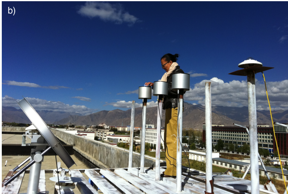
Figure 3.2: (a): Satellite picture of the instrument location in Lhasa and the distances from the instrument to the mountains nearby. (Google Earth image taken on 02/10/2015. Map data: Centre National d'Etudes Spatiales (CNES) 2015 distribution Astrium services, spot image.) (b): Instruments mounted at Tibet University in Lhasa: three NILU UV radiometers acquires UV measurements are placed close to the pyranometer. On the left side of the figure, a pyranometer with a shadow band is placed to detect diffuse light. Source: Norsang Gelsor, 2013.
