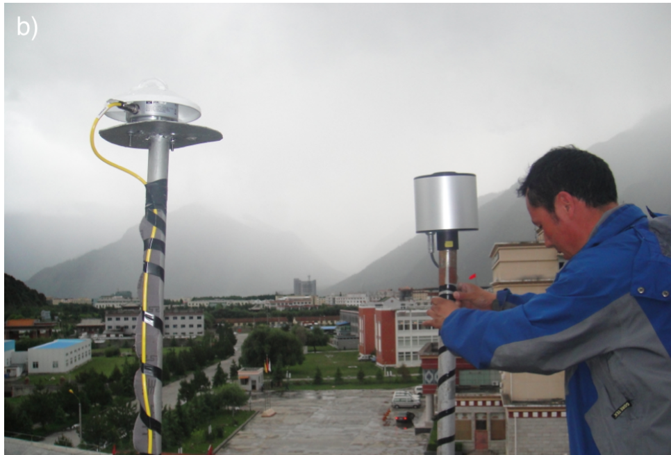
Figure 3.6: (a): Satellite picture of the instrument location in Nyingchi and the distances from the instrument to the mountains nearby. (Google Earth image taken on 13/01/2015. Map data: Google, DigitalGlobe and CNES 2015 distribution Astrium services spot image.) (b): Instruments at the Nyingchi site: a NILU UV radiometer and a pyranometer are mounted together to record UV measurements and broad-band irradiance data, respectively. Source: Norsang Gelsor, 2013.
