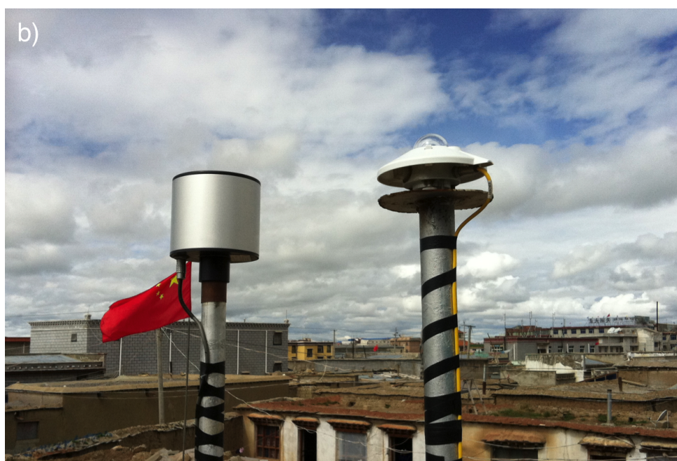
Figure 3.3: (a): Satellite picture of the instrument location in Nagchu and the distances from the instrument to the mountains nearby. (Google Earth image taken on 21/12/2011. Map data: Google, DigitalGlobe.) (b): Instruments mounted in Nagchu site: a NILU UV radiometer and a pyranometer are mounted next to each other, the NILU instrument records UV measurements and the pyranometer recording broad-band irradiance data. Source: Norsang Gelsor, 2013.
