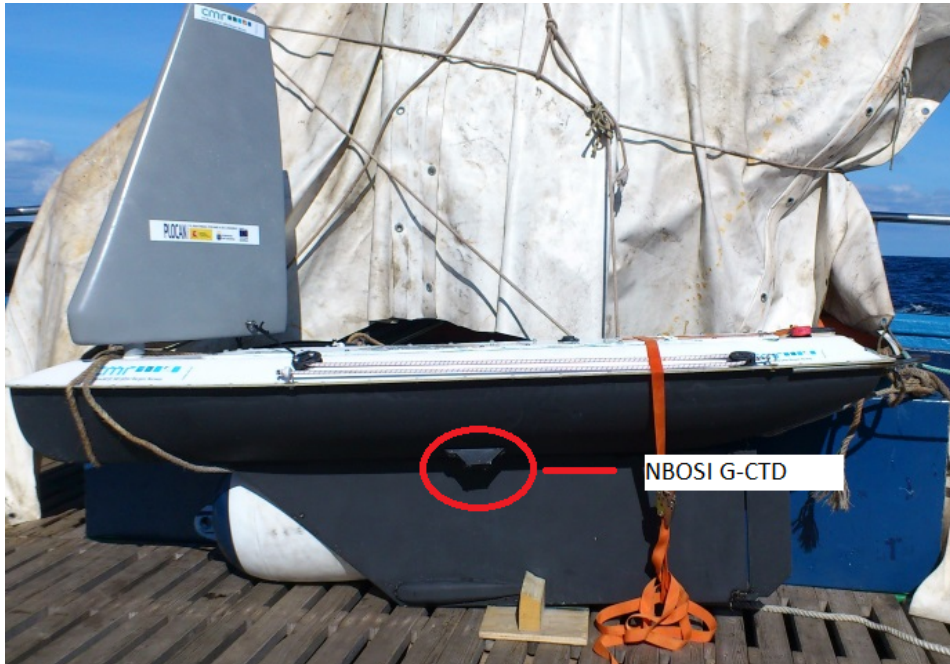
Figure 3.3: NBOSI G-CTD equipped on the Offshore Sensing SailBuoy ( www.sailbuoy.no ).
