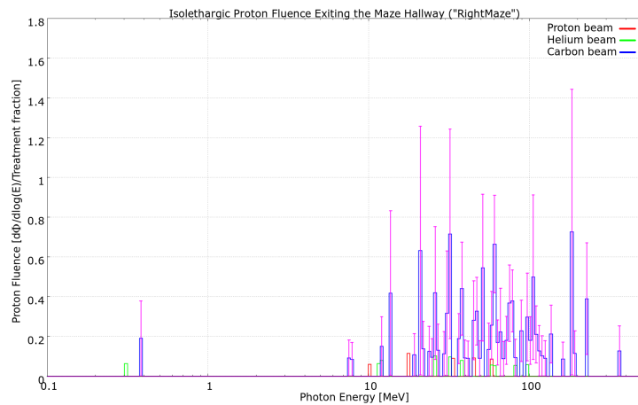
(c) Isolethargic differential fluence plot of protons exiting the maze hallway in simulation setup "RightMaze".
