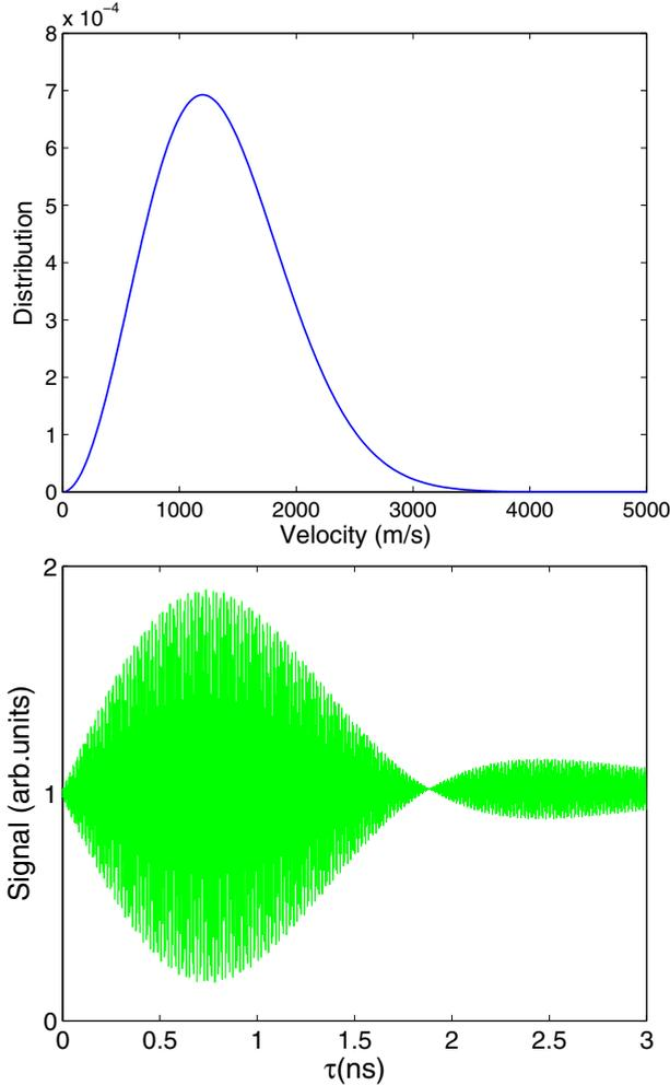
FIG. 3. (Color online) Upper panel: Thermal distribution of velocities of lithium atoms for  $T = 600$  K according to Eq. (17). Lower panel: Signal that will be detected in the case of velocity distribution displayed in the upper panel. The crossing angle  $\theta = 20^\circ$  and laser pulse parameter  $\alpha = 10^{26} \text{ s}^{-2}$ . The oscillations are a result of sampling frequency; the real inner oscillations are faster with frequency  $\omega_g$ .
