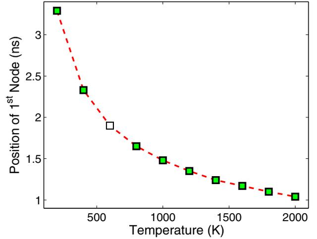
FIG. 4. (Color online) The expected position of the first node in the signal of Ramsey fringes as a function of temperature, when considering the thermal distribution of velocities given by Eq. (17). The white square corresponds to the node from Fig. 3.
