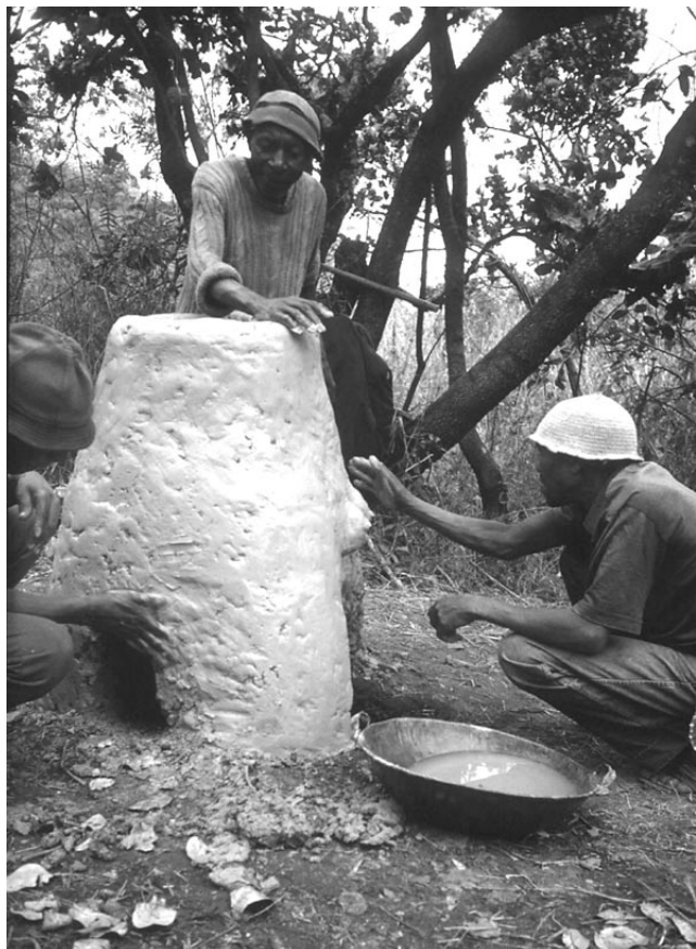
Figure 3. The Pangwa smelting furnace, liteende (photo by Randi Barndon)
