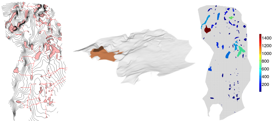
Fig. 1. Structural traps in the Statfjord formation. Left : Topographic map of caprock, with traps and spill paths. Middle : 3D plot with largest trap and associated spill region highlighted. Right : Traps coloured according to CO 2 storage capacity (megatonnes).
