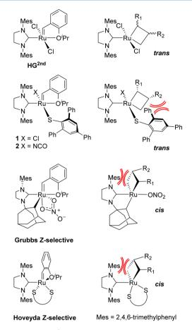
**Figure 1.** Positioning (*cis* or *trans* with respect to the NHC ligand) of the metallacyclobutane moiety in the catalytic cycle of the Hoveyda–Grubbs second-generation catalyst and of various Z-selective ruthenium-based catalysts.
