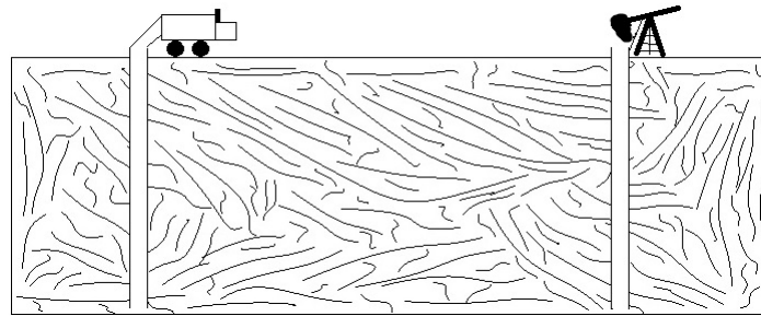
Figure 2.2.1 General diagram of the MEOR technique in an oil reservoir. On the left well, bacteria and nutrients are injected, meanwhile the oil is extracted on the right well. Inside the reservoir, the bioproducts change the properties of the porous medium and fluids, allowing to increase the production.
