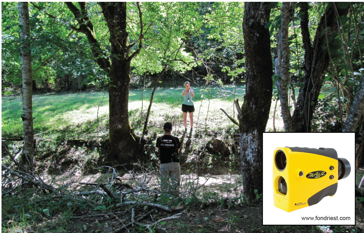
Fig. 10: Profiling by the use of a laser rangefinder gives highly accurate measurements of distance. The instrument (lower right corner) is pointed towards a reflective surface (e.g. a face, as shown here) and the reflection of the laser beam provides measurements of direct, horizontal and vertical distance, as well as azimuth and inclination.
