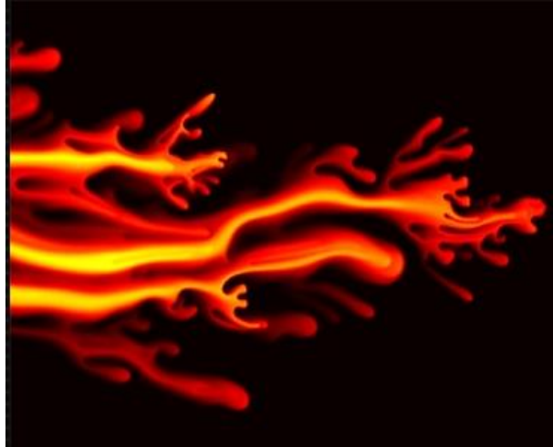
Figure 10: Illustration of viscous fingering due to an unfavorable mobility ratio. The figure shows an unstable displacement process of a more viscous fluid (dark) by a less viscous fluid (light). Figure from (Jha, 2011)
