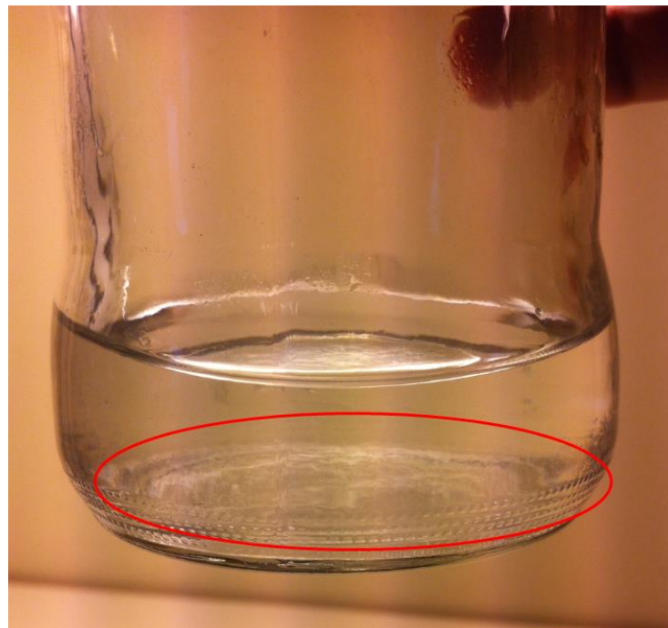
Figure 48: Precipitation of calcite particles in the production flask. This was observed at the end of several experiments.
