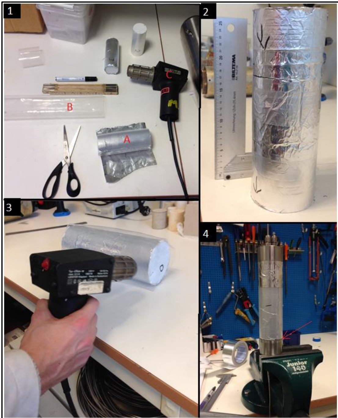
Figure 17: Wrapping procedure. 1) A – fractured core tightly wrapped in aluminum foil. B – shrinking sleeve. C – heating pistol. 2) Aluminium foil was used to wrap the core and keep the pieces in place. 3) Shrinking sleeve is used as additional wrapping stability. A heating pistol was used to shrink the sleeve so that it would attach to the aluminum wrapped core. It was important to evenly distribute heat to the entire shrinking sleeve to prevent it from folding or any other shrinking irregularities. 4) Inlet and outlet endpieces of the coreholder was connected to the prepared cored with aluminum tape before placing the core into the core holder to ensure that injected fluids flow through the core and not around it (on the outside). The red arrow points at the open space between an endpiece and the core that potentially could cause fluid flow around the core if not connected with aluminum tape.
