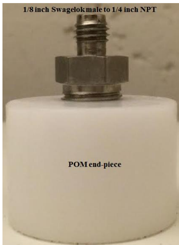
Figure 7.2: Inlet POM end-piece with 1/8 inch Swagelok male to 1/8 inch NPT. The outer diameter was 35 mm and the inner diameter was 22.5 mm.
