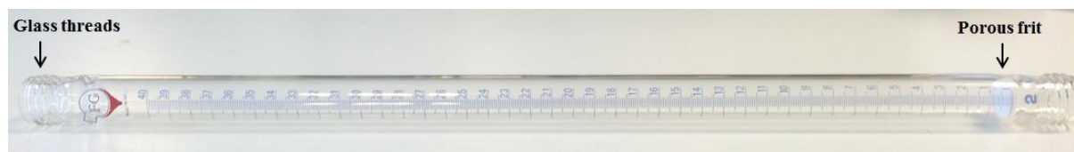
Figure 7.1: Glass cylinder with centimeter scale and fitted porous frit. The length was 50 cm and inner diameter was 20.4 mm.
