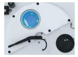
Figure 2.5: Picture of Windcube V1 wiper. Adapted from Pauliac (2009)
