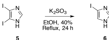
Scheme 14 One-step synthesis of 4(5)-Iodo-1 H -imidazole ( 6 ) from 4,5-diiodo-1 H -imidazole ( 5 )
