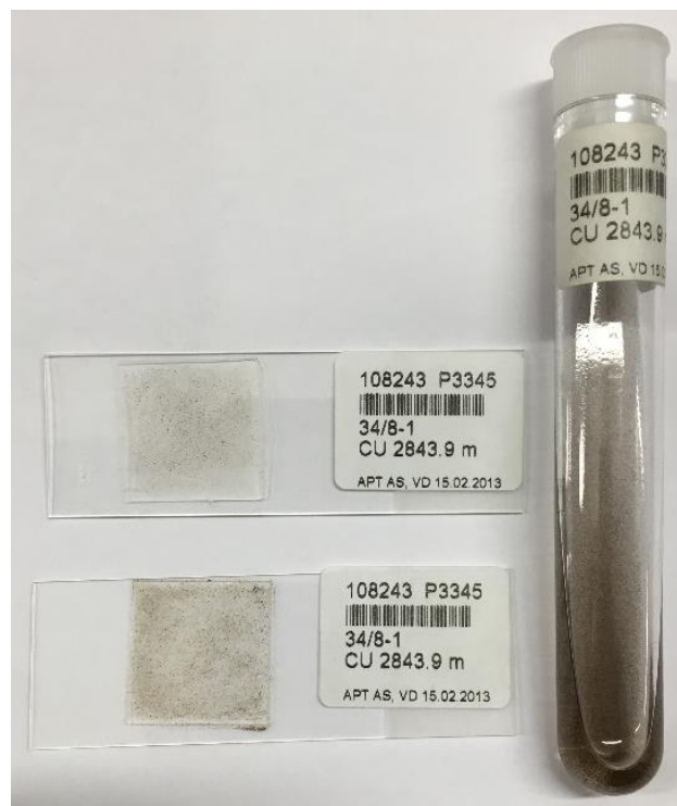
Figure 13: Showing two prepared palynological slides and a sample tube with final aqueous residue (mount residue). Processed during “preparation of slide” course at Applied Petroleum Technology, Lillestrøm.
