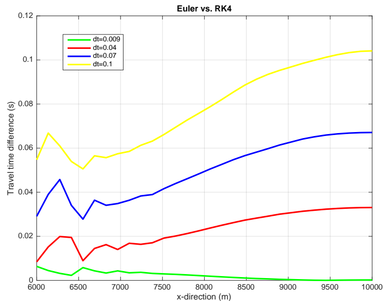
Figure 68: Travel time differences for Euler's method vs. fourth order Runge-Kutta as computed using the 1D velocity model.
