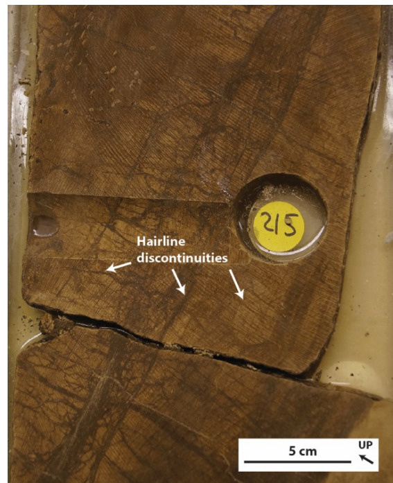
Figure 5.5: The sampling location in well 30/9-B- 44B for thin section H215 at 4305.50 m MD. This thin section contains the deformation band studied by Wennberg et al. (2013). Notice discontinuities subparallel to and with high angles to the bedding, named “hairline discontinuities”, also referred to as “hairline fractures” in the literature (Feazel, 1988). The arrow indicate the orientation to the bedding relative to the direction up towards the sea floor.
