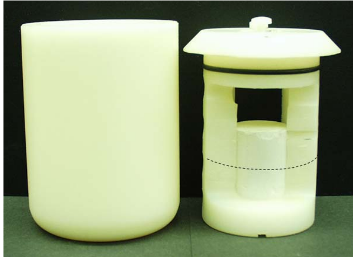
Figure 5.2.1.2: The centrifuge core holder. The free water level is indicated by the stippled curve. Octadecane was surrounding the plug above this curve.
