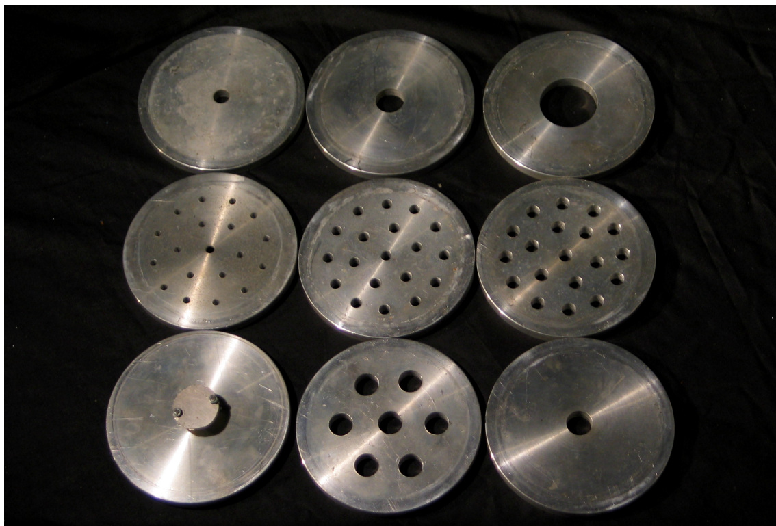
Figure 4.2 A selection of some of the orifices used. The aluminum disk in the lower left corner has a small piece of metal mounted 10 mm away from the orifice opening to redirect the flow in a radial manner. Number of orifices in the discs is 1, 7 and 19.
