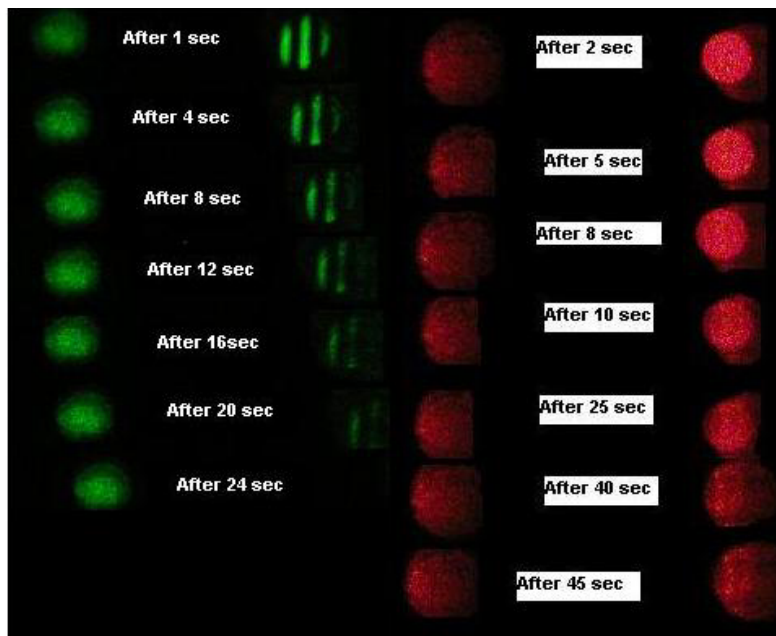
Figure 26 The virtual images (holograms) are the ones to the right. These disappear gradually, due to thermal back-conversion. The reduced reference beam is the one to the left for both lasers.
