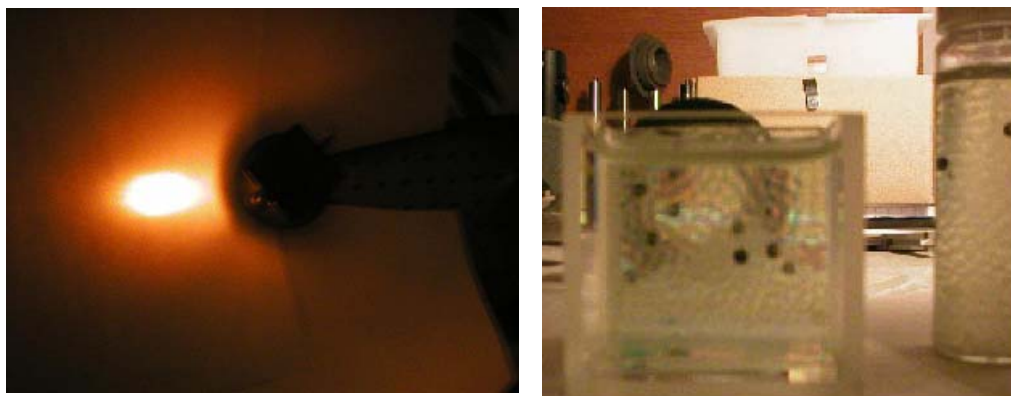
Figure 22 Transmitted and scattered light through particles in fluid, seen from above to the left. A glass container in white light conditions (notice the black tape behind it) is displayed in the image to the right.
