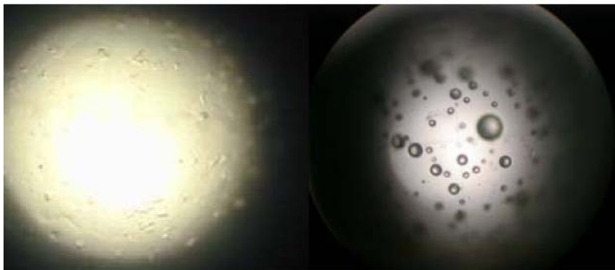
Figure 19 Two particles types that was evaluated for use in the experiment. Left particle is 2mm and the one to the right is 0,5mm in diameter.
