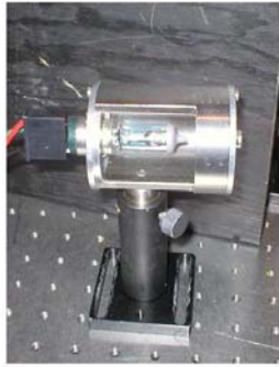
Figure 30 The design for a reflector made of a metal tube, to converge the light beam and prevent stray light.
