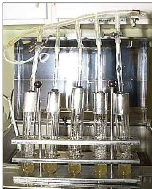
Figure 4.25: Preliminary construction of the Bioassay implemented the use of air to provide mixing.
