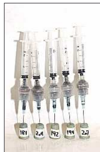
Figure 3.5: Syringe assemblage for SEM preparations.
