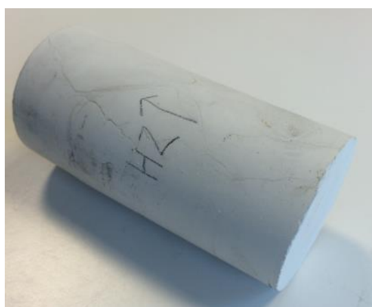
Figure 10 – Core plug H2 drilled from outcrop MM4-5, collected from location Pinapple Steps in Eastbourne England. Core diameter is 4.96 cm (2") and core length is 10.01 cm. Figure shows several fractures visible.
