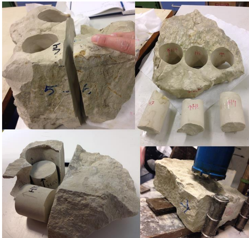
Figure 11 – LRQC core plugs being drilled from outcrops of six different zones described in Figure 5. Right top: Three horizontal cores; H7, H2 and H9 drilled from outcrop MM3-4. The outcrop has visible colour differences. Left top: Outcrop from zone MM5-6 cut in half. Vertical core plugs drilled from the one to the left, while horizontal core plugs are drilled from the one to the right. The outcrop show colour variation and have visible heterogeneities. Right bottom: The bit (in blue) is about to drill a core plug from BED 5. Left bottom: The two core plugs, H10A and H10B drilled from zone BED 5. One is horizontal and one is vertical. Photos are taken by Dr. Marianne Steinsbø, Department of Physics and Technology, UoB.
