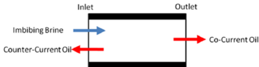
Figure 43 – Boundary conditions and direction of flow during the TEOFSI test. Inlet end is in contact with brine, while outlet end is in contact with oil. Brine can only imbibe from the end in contact with brine, while oil can be produced from either or both ends (Haugen et al., 2014).
