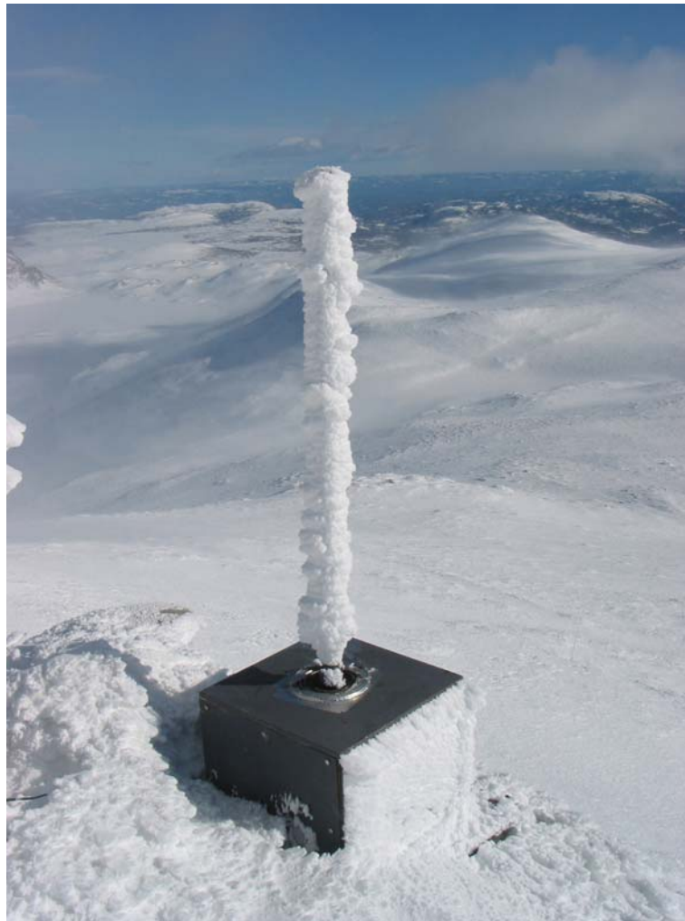
Figure 5. Ice accretion on the ice scale April 1, 2003. The length of the rod is 1 m, and the diameter without ice is 3 cm.
