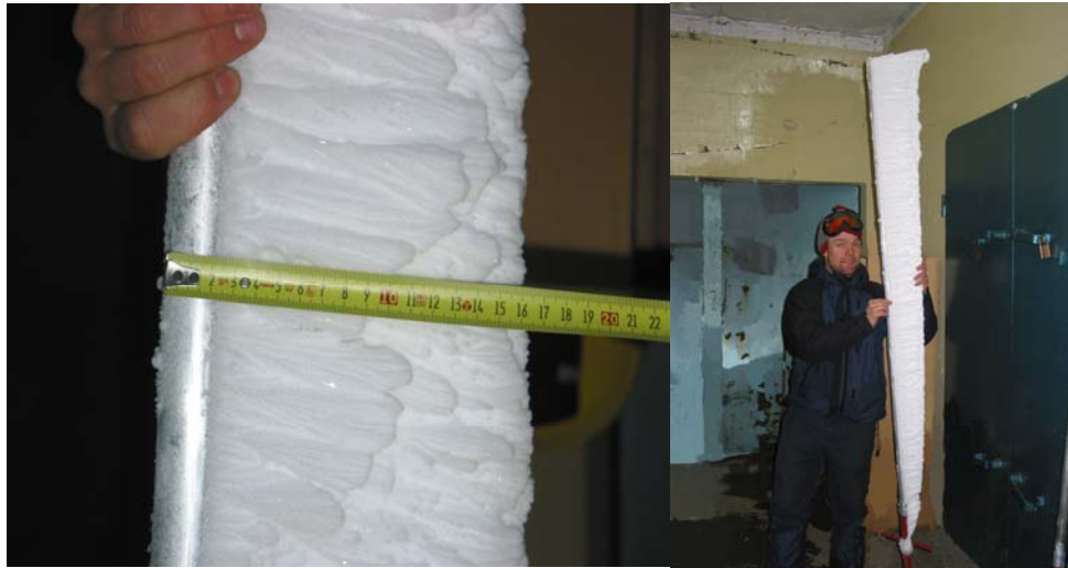
Figure 4. Measurements of the length of the ice wane to the left, and a demonstration of a typical ice accretion on a stick to the right.
