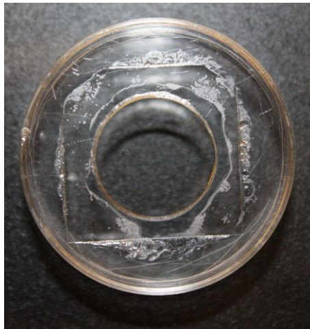
Figure 36: Cover slip mounted on a petri dish using grease. [1] This was done to be able to add an aqueous solution on the coverslip.
