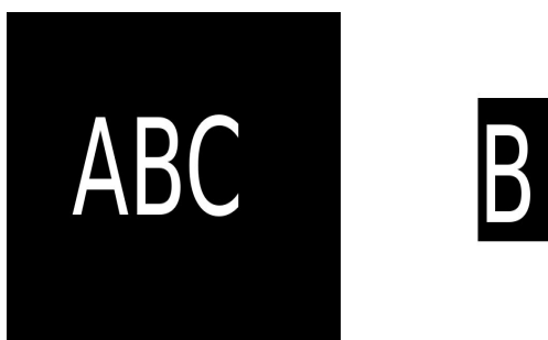
Figure 2.1: Image and Template. Cross correlation finds the area in the image in which the template fits best.
